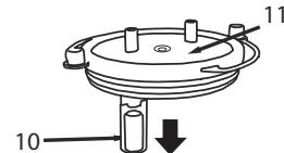
2. Remove the float (.10a) from the safety device (.10)
