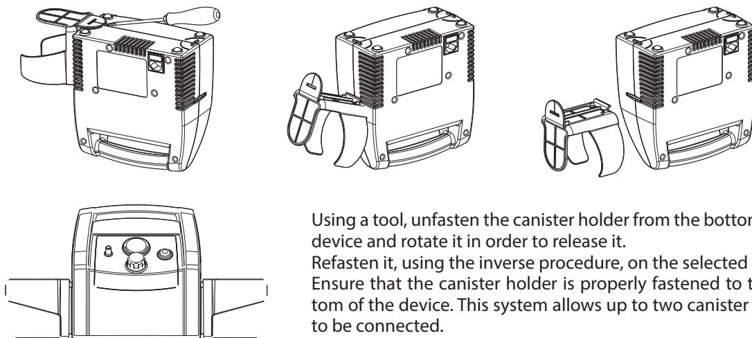
Using a tool, unfasten the canister holder from the bottom of the device and rotate it in order to release it.
