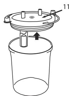
1. Remove the safety device (.10) from the canister lid (.11)
