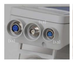
[2] Plug the probe in the corresponding connection
