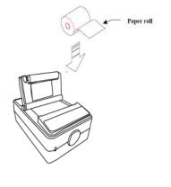
2.Feed the end of the paper roll through the printer cover and close the cover. The printer is ready to print.
