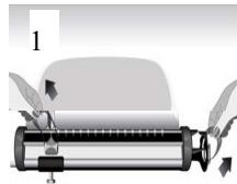
**Pictogram 1: Remove transport security of sliding Weights and Sliding weight bar.**
