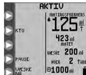
Figure 15A. RUNNING mode screen for continuous feed mode.
