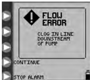
Figure 29. Flow Error screen.
