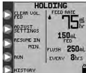
Figure 18A. HOLDING mode options, continuous feeding mode.
