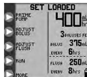
Figure 7D. Opening menu for Intermittent Feed mode with a feed & flush set.
