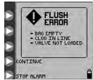
Figure 28. Flush Error screen.
