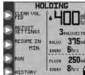
Figure 18B. HOLDING mode options, intermittent feeding mode.
